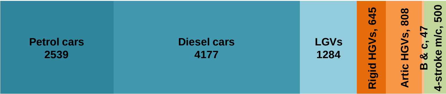
Figure A.3 – Schematic illustration of the relationship between traffic composition and route type, comparing the breakdown by vehicle type for NAEI 12 Eng[3] U15 and NAEI 12 Eng[3] M15 route types for an example AADT of 10000 vehicles per day.
